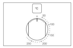
Each oven has its own temperature selector. Select the appropriate temperature for the food to be cooked. The temperature can be freely selected within the given range.
